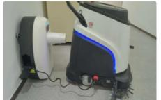
(3) Observe the machine screen displaying a charging plug icon to confirm that the robot is being charged.
