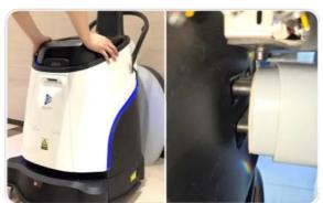
(3) Push the machine until the automatic charging interface appears on the machine's screen.
