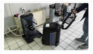
(3) Open the protective soft rubber on the right side of the squeegee cover, align the charging plug with the charging port, and insert it.
