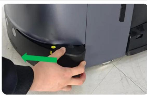
Note: It is forbidden to directly turn off the boat switch when robot is on. Before turning off the boat switch, it is necessary to use the button on the top cover to turn off the machine first.
