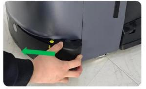
Note: It is forbidden to directly turn off the boat switch when robot is on. Before turning off the boat switch, it is necessary to use the button on the top cover to turn off the machine frist.
