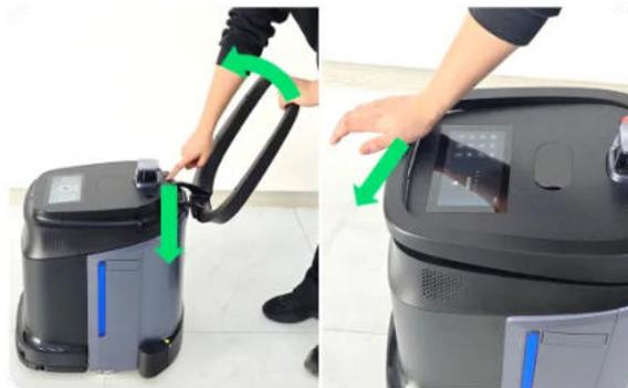
(3) Click the "Manual Mode" button on the machine screen; rotate the machine and align the charging electrode plates of the machine with those of the charging pile.
