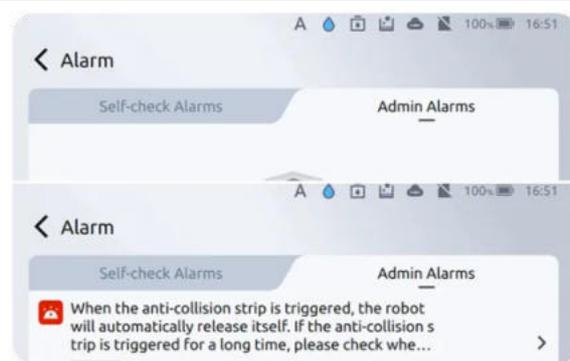
(3) When the machine triggers an abnormal alarm, there will be a red pop-up at the bottom of the screen. Click "View Details" to quickly check the alarm information.
