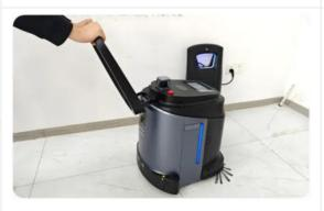
(3) Click the "Manual Mode" button on the machine screen; rotate the machine and align the charging electrode plates of the machine with those of the charging pile.
