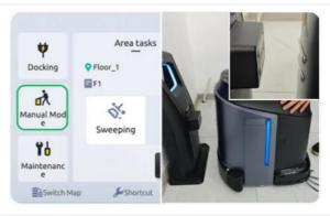
(7) Push the machine to make the charging electrode plates of the machine contact with those of the charging pile or workstation, and release your hands when the light strips of the machine and the charging station turn green.
