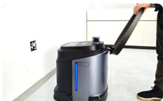
(4) When the screen displays a "positioning success" message and you can hear the machine's voice prompt saying "Positioning successful," it indicates that the machine has successfully completed the initial positioning.
