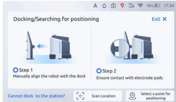
(5) Manually push the machine to the charging pile or workstation. Press the unlock button on the handle, push the handle forward at the same time, and finally press down to lock the handle.
