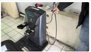
(4) While charging, the robot's light strip shows green; after charging is complete, rotate the blue fixed ring of the charging plug counterclockwise and pull out the charging plug outward at the same time.
