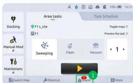
(2) If the machine is operating normally, there will be no alarm messages; if there is an abnormality with the machine, alarm messages will appear.
