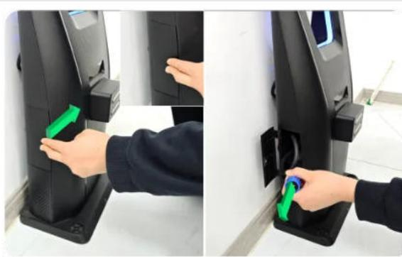
(4) While charging, the robot's light strip shows green; after charging is complete, rotate the blue fixed ring of the charging plug counterclockwise and pull out the charging plug outward at the same time.
