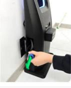
(4) While charging, the robot's light strip shows green; after charging is complete, rotate the blue fixed ring of the charging plug counterclockwise and pull out the charging plug outward at the same time.
