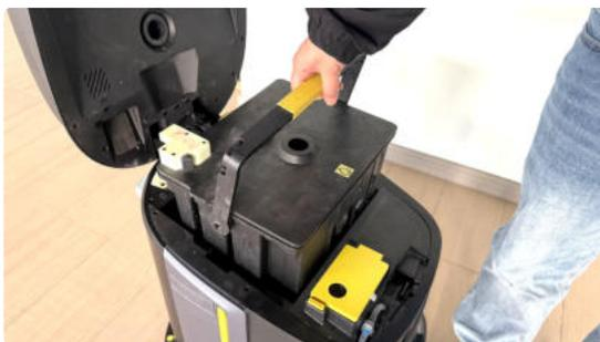
(3) Open the sewage tank cover, remove the filter basket, and then pour out the waste water.
