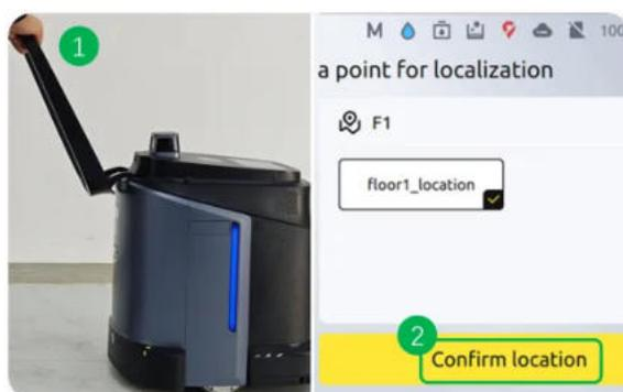
(8) When the screen displays a "positioning success" message and you can hear the machine's voice prompt saying "Positioning successful," it indicates that the machine has successfully completed the initial positioning.
