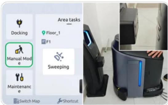
(4) Push the machine to make the charging electrode plates of the machine contact with those of the charging pile until the light strips of the machine and the charging pile turn green.
