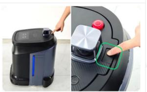
(3) Turn up the handle to the maximum angle and push the machine manually.
