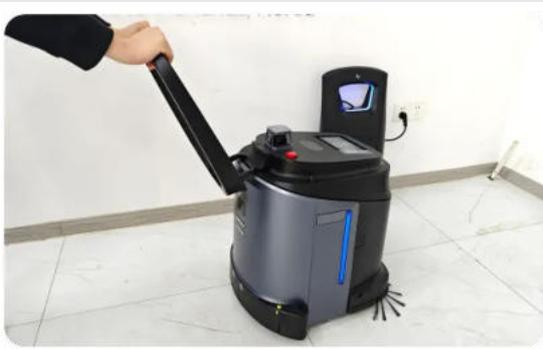
(3) Open the protective soft rubber on the right side of the squeegee cover, align the charging plug with the charging port and insert it.
