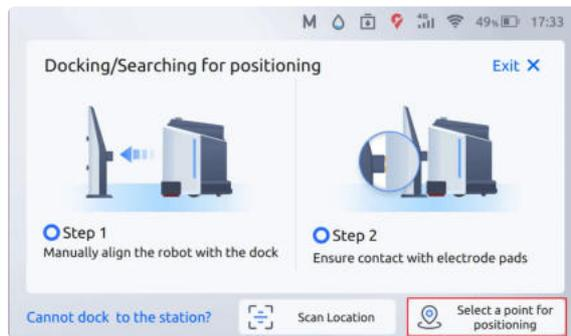
(5) Select the positioning point. (The positioning point is set in advance when the robot is deployed.)
