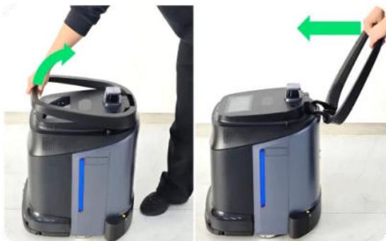
(4) Press the unlock button, then push the handle forward, and finally press down to lock the handle.
