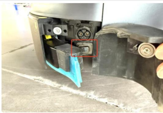
(3) Reinstall the protective soft rubber on the right cover of the squeegee. Press and hold the power button on the top of the machine for several seconds until the display screen lights up.
