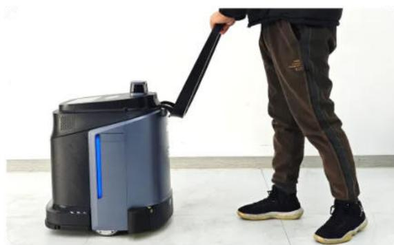
(3) Align the drain port of the machine with the floor drain, turn on the switch of the drain port downward, and start to empty the clean water.
