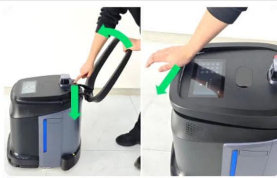
(3) Click the "Manual Mode" button on the machine screen; rotate the machine and align the charging electrode plates, water refilling inlet, and drainage outlet with the workstation's charging electrode plates, water refilling rod, and wastewater tray, respectively.
