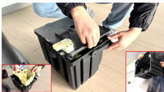
(4) Reinstall the filter basket and the sewage tank cover, reinsert the sewage tank and close the head cover.
