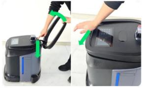
(3) Click the "Manual Mode" button on the machine screen; rotate the machine and align the charging electrode plates, water refilling inlet, and drainage outlet with the workstation's charging electrode plates, water refilling rod, and wastewater tray, respectively.
