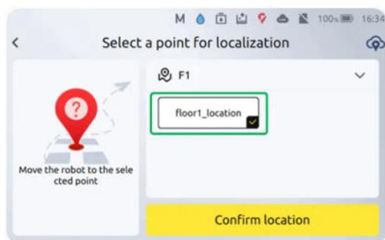
(6) ① Manually push the machine to the actual position where the positioning point is located. ② Click "Confirm location" after arrival.
