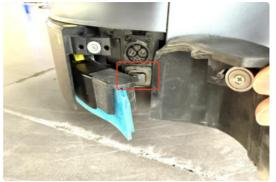
(3) Reinstall the protective soft rubber on the right cover of the squeegee. Press and hold the power button on the top of the machine for several seconds until the display screen lights up. (4) After entering the password, click Login.
