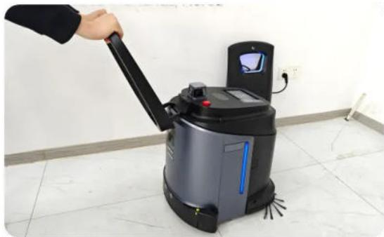
(2) Press the unlock button, then push the handle forward, and finally press down to lock the handle.
