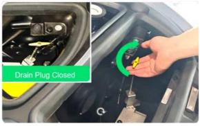
(8) Close the drain pipe cap and retract the drain pipe.
