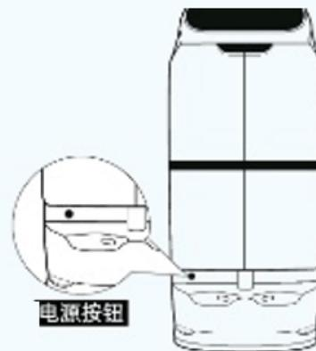
The power button is at the bottom of the robot.
